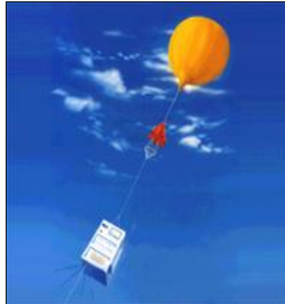
Radiosond instrument attaced to a balloon
